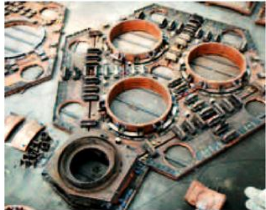
Metix's use of copper for the roof sections of closed furnaces significantly improves the cooling performance and, because welding is completely avoided, cracking and leaking is prevented.
