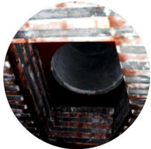
Between the cooling channels, which are 100 mm apart, dovetails are cast into the inside surfaces of the copper and filled with refractory material. This prevents the refractory from falling off the underside of the roof and ensures that the cooling efficiency does not degrade with time.
